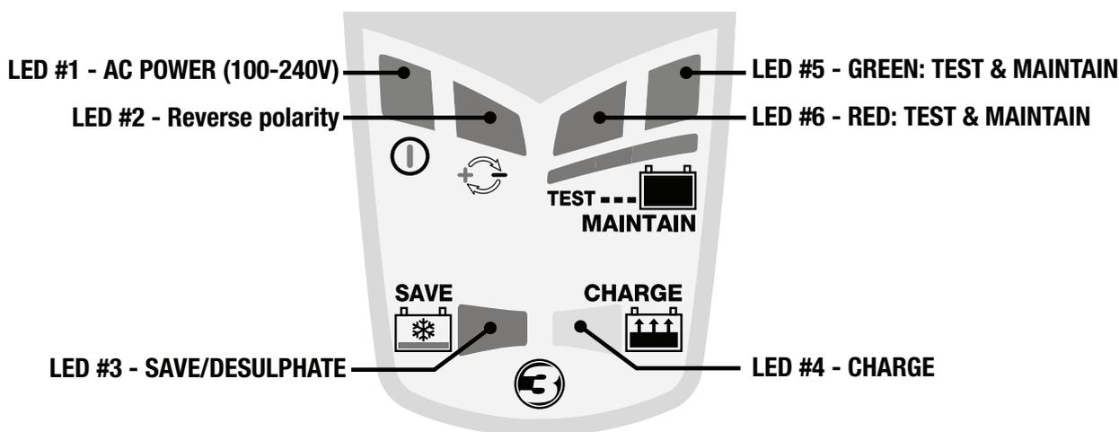
**1. LED #1 - Power on. Confirms AC power supply to the charger. Light intensity is low during POWER SAVING MODE.**
